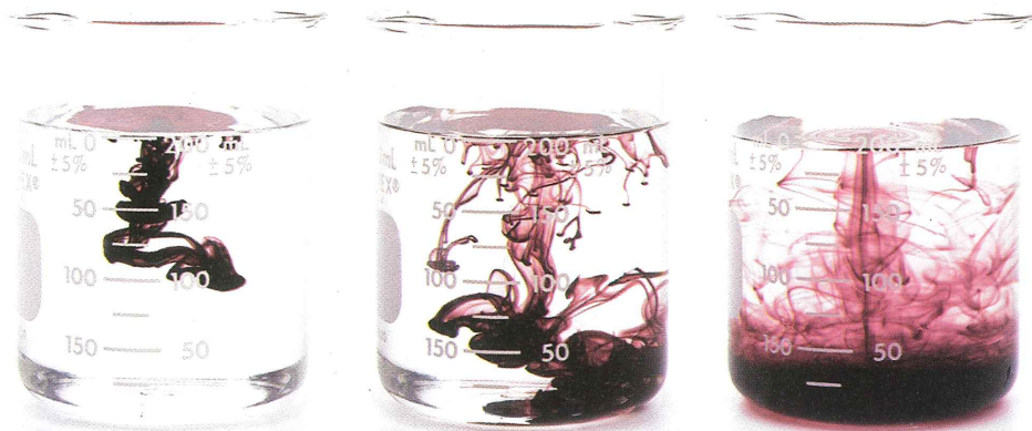
Figure 2.2 In time, the ink particles will become evenly dispersed with the water particles, and the whole solution will appear ink-coloured.
